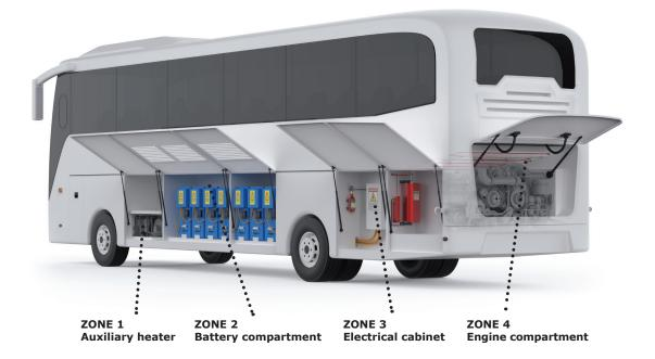
The different protection zones are then protected in various ways by robust detection and suppression systems – both liquid based and gas-based solutions.
